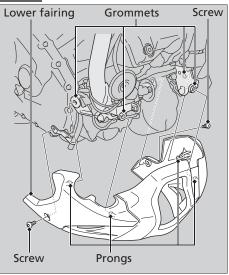
The lower fairing must be removed to service the coolant reserve tank and spark plugs, to replace the engine oil filter.
