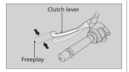
Check the clutch cable for kinks or signs of wear. If necessary have it replaced by your dealer.
