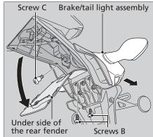
**5.** Turn the socket counterclockwise, and remove it.
