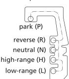
You should move the shift select lever only when the vehicle is stopped with your foot on the brake pedal and with the engine idling. Use a firm motion to select the appropriate gear. Have your vehicle checked by a dealer if you experience any shifting problems.
