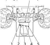
The spring pre-load adjuster has 5 positions for different load or driving conditions. Before adjusting the spring pre-load, jack up your Honda SXS (page 144) to avoid damaging the adjusters.
