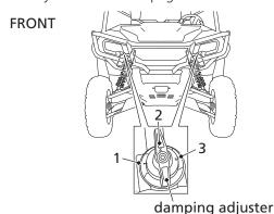
The damping adjuster has 3 positions for different load or driving conditions
