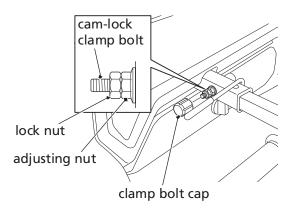
Do not apply a grease or lubrication to the handhold slider surface and cam-lock clamp.
