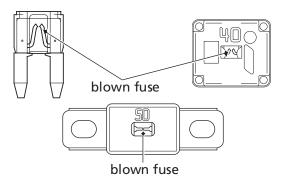
Check all the fuses before looking elsewhere for another possible cause of the problem. Replace any blown fuses and check component operation.
