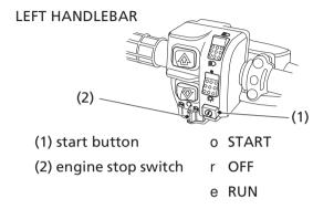
The start button (1) is used for starting the engine. Pushing the button in starts the engine. See *Starting Procedure*, page 52.
