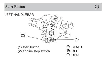
The start button (1) is used for starting the engine. Pushing the button in starts the engine. See *Starting Procedure*, page 51.
