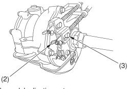
(2) brake pedal adjusting nut
