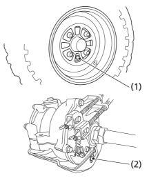
(1) front brake inspection hole plug
