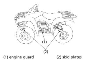
The engine guard (1) protects the engine crankcase. The skid plates (2) protect the frame and rear final gear case. Check the guard and plates for cracks, damage or looseness at intervals shown in the Maintenance Schedule.
