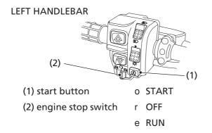
The start button (1) is used for starting the engine. Pushing the button in starts the engine. See *Starting Procedure*, page 51.
