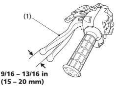
(1) rear brake lever/parking brake lever
