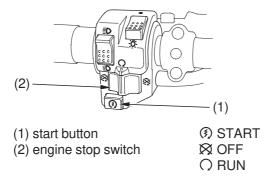
The start button (1) is used for starting the engine. Pushing the button in starts the engine. See *Starting Procedure*, page 49.
