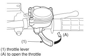
The throttle controls engine rpm (speed). To increase engine rpm, press the throttle lever (1) with your thumb. To reduce engine rpm, release pressure on the throttle lever. The throttle will automatically return to the closed position (engine idle) when you remove your thumb.
