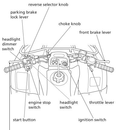
rear brake lever/parking brake lever
