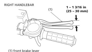
1. Measure the distance the brake lever moves before the brakes start to take hold. Freeplay, measured at the tip of the front brake lever (1) should be:
