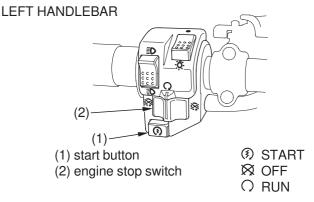
The start button (1) is used for starting the engine. Pushing the button in starts the engine. See *Starting Procedure*, page 47.
