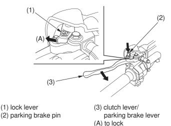
The lock lever (1) and parking brake pin (2) on the clutch lever/parking brake lever (3) allows it to be used as a parking brake. To operate, push down and hold the parking brake pin, squeeze the clutch lever/parking brake lever and then lock it with the lock lever. See *Parking* page 70.
