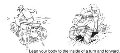
To make a turn on level ground: Steer the handlebar and lean your body toward the inside of the turn. Leaning helps balance the vehicle, and it
