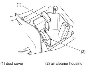
Do not push the dust cover (1) too far into the air cleaner housing (2). If the dust cover is dirty, clean it.
