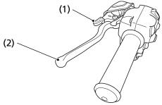
(1) parking brake lock lever(2) rear brake lever/parking brake lever
