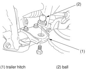
The trailer hitch (1) is located on the rear end of the rear frame. To use the hitch, you'll need a proper size ball (2) as specified by the trailer manufacturer.
