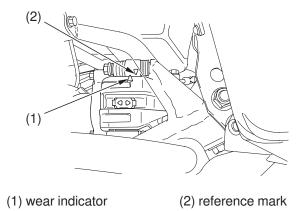
Check the wear indicator. If the wear indicator (1) aligns with the reference mark (2), replace both pads as a set, see your dealer for this replacement.
