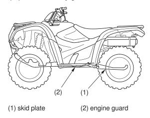
The skid plate (1) protects the rear final gear case. The engine guard (2) protects the frame and engine crankcase. Check the skid plate and engine guard for cracks, damage or looseness. Tighten any loose fasteners. Replace the skid plate or engine guard as required.
