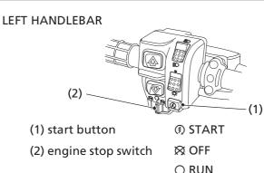
The start button (1) is used for starting the engine. Pushing the button in starts the engine. See *Starting Procedure*, page 73.
