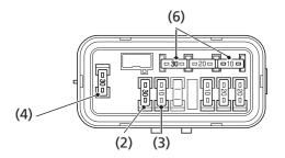
(2) main fuse 1(3) main fuse 2(4) shift motor fuse
