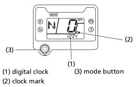
After the battery is reconnected (page 184), check the clock. Readjust the clock if necessary.
