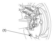
(1) rear brake drain bolt
