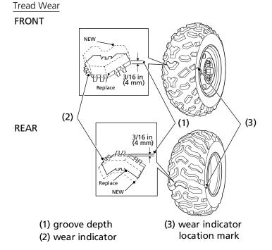
To check the condition of a tire tread, measure the groove depth (1) in the center of the tire, or check the wear indicator (2). For best performance, you should replace a tire before the tread depth at the center reaches the following limits:
