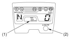
(1) tripmeter (2) hourmeter/odometer/tripmeter select button
