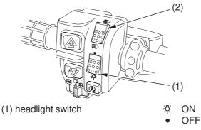
The headlight switch (1) is used to turn the headlight ON ( $\stackrel{*}{x}$ ) or OFF ( $\stackrel{\bullet}{\bullet}$ ). To operate, turn the switch to ON ( $\stackrel{*}{x}$ ) or OFF ( $\stackrel{\bullet}{\bullet}$ ).
