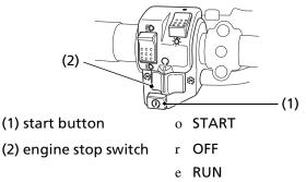
The start button (1) is used for starting the engine. Pushing the button in starts the engine. See *Starting Procedure*, page 73.
