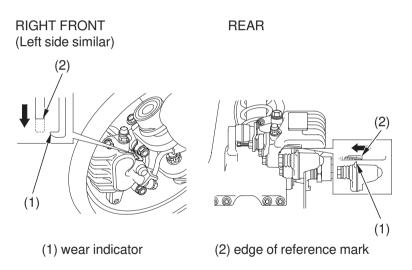
Check the wear indicator (1). If the wear indicator aligns with the edge of the reference mark (2), both pads must be replaced, see your dealer for this replacement.
