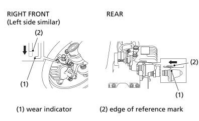
Check the wear indicator (1). If the wear indicator aligns with the edge of the reference mark (2), both pads must be replaced, see your dealer for this replacement.
