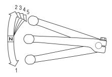
The shift lever is located near the left footpeg. One full stroke of the shift lever shifts the transmission to the next higher or lower gear in the shifting sequence. The shift lever automatically returns to the horizontal position when released.
