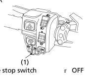
(1) engine stop switch r OFF e RUN
