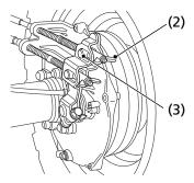
(2) brake lever adjusting nut(3) brake arm pin
