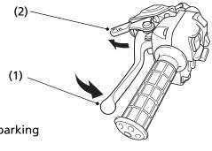
(1) rear brake lever/parking brake lever
