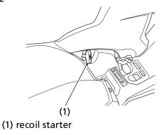
The recoil starter (1) is used to start the engine when the battery is low. See Using the Recoil Starter (Canada only), page 84.
