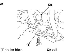
The trailer hitch (1) is located on the rear frame. To use the hitch, you'll need a proper size ball (2) as specified by the trailer manufacturer.
