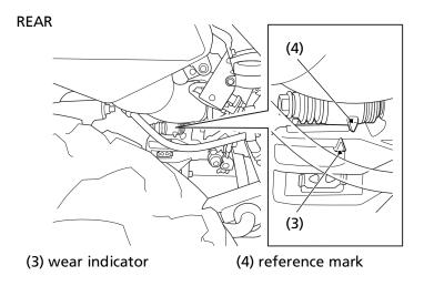
Check the wear indicator. If the wear indicator (3) aligns with the reference mark (4), replace both pads as a set, see your dealer for this service.
