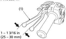
(1) rear brake lever/parking brake lever
