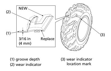
To check the condition of a tire tread, measure the groove depth (1) in the center of the tire, or check the wear indicator (2). For best performance, you should replace a tire before the tread depth at the center reaches the following limits:
