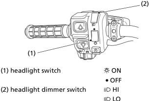
The headlight switch (1) is used to turn the headlight ON ( $\mathfrak{P}$ ) or OFF ( $\bullet$ ). To operate, turn the switch to ON ( $\mathfrak{P}$ ) or OFF ( $\bullet$ ).
