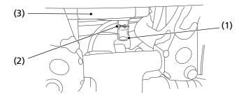
(1) drain tube(3) air cleaner housing(2) clip
