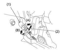
(1) rear brake light switch (2) adjusting nut
