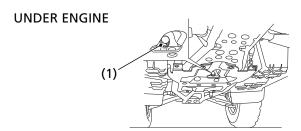
(1) engine oil drain bolt
